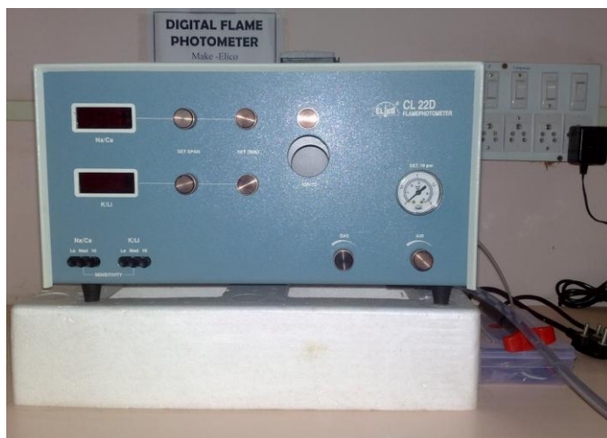
Figure 1 Flame photometer (Make-Elico-Model-CL220)
